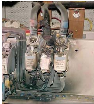
Fig. 9: Fuse exploded due to resonances.
