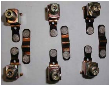
Fig. 3: Burnt main contacts of a capacitor contactor.
